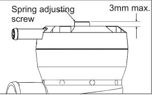
Unlike an atmosphere-venting BOV, the spring pre-load on the Mach 2 does not need to be adjusted to prevent stalling or backfiring, since all of the vented air is recirculated in the same way as the OEM bypass valve.
