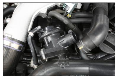
3) Fit the GFB Mach 2 value to the mounting flange, making sure the supplied red o-ring is fully inserted into the groove in the underside of the GFB value as shown below. Replace the two bolts, vacuum and recirc hoses and clamps.
